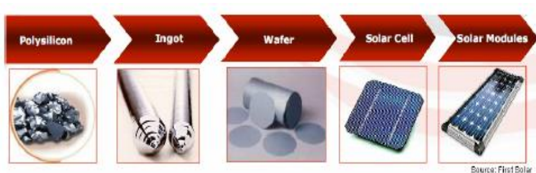
Figure 124: Stages in PV manufacturing process
